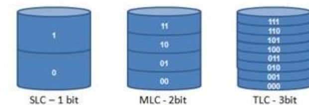
Pic. 1 Single-level cell (SLC) memories come with two states (0 or 1), multi-level cell devices (MLC) come with four states, and triple-level cell (TLC) components come with a critical total of eight possible states
